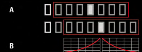
A: two consecutive time points showing how neighboring frames (red box) are used on a rolling basis for improving the SNR of the central frame (filled box) B: additional parameter allows to define how neighboring frames are weighted, less weight means less influence, and less motion blurring.
